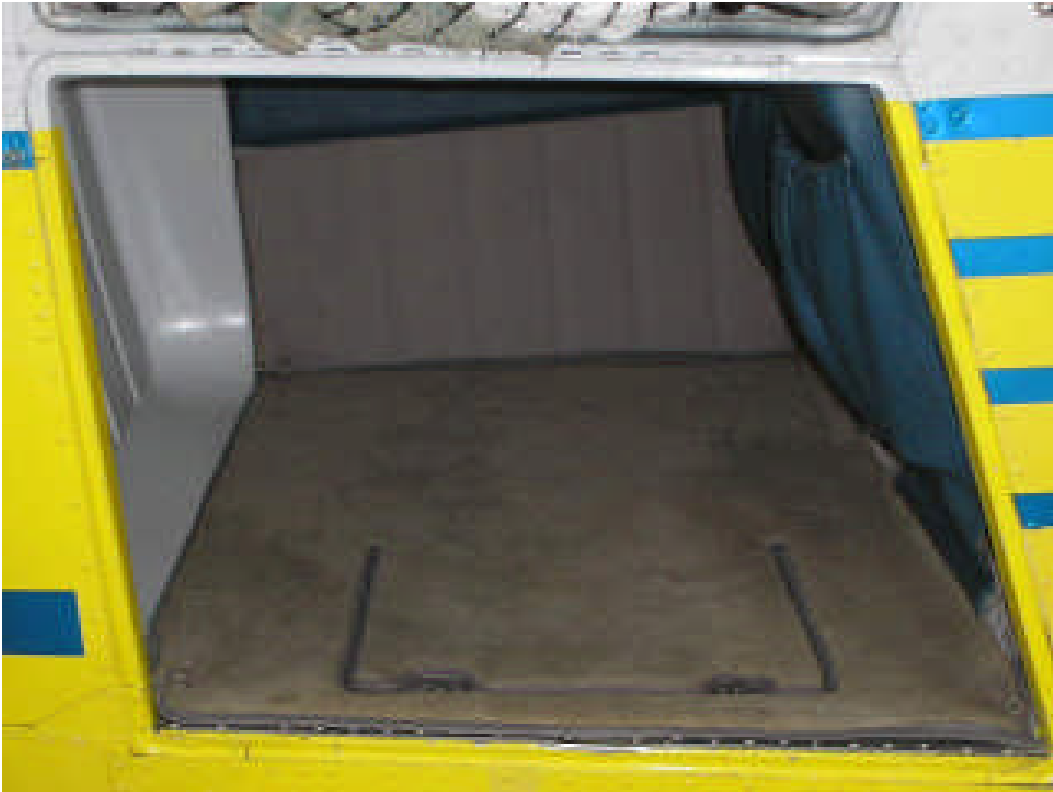
Aft baggage door opened showing baggage compartment mounted below the floor and concealed by the carpet.
